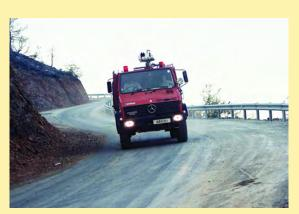
engines which are posted at the various forest stations. Most of them are 4X4 vehicles ready to be driven on off-road conditions in order to be used in fire fighting. The Department also is equipped with a number of small fire engines which are mainly used for patrolling and rapid intervention in case of fire.
